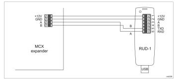
Fig. 3 Connection of the expander to RUD-1 interface (firmware update)
