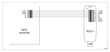
Fig. 1 Connection of the expander to RUD-1 interface (configuration)
