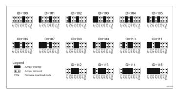
Fig. 2 Manual addressing of MCX8-BRD expander
