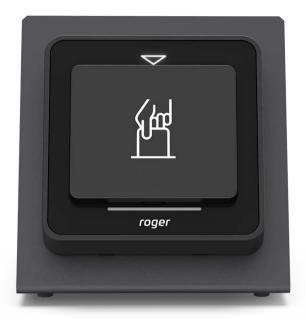
RUD-4-DES is a desktop reader and writer for MIFARE® Classic, Plus (S, X) and DESFire (EV1, EV2) cards which also allows reading an EM 125 kHz standard proximity cards. It is supplied directly from a USB serial port, which is also used for communication with the PC. The device has a stable metal desktop stand with a card holder. The RUD-4-DES can be used as a card enrol reader for the access control system or any other application which requires a card reader. A card can be enrolled straight
