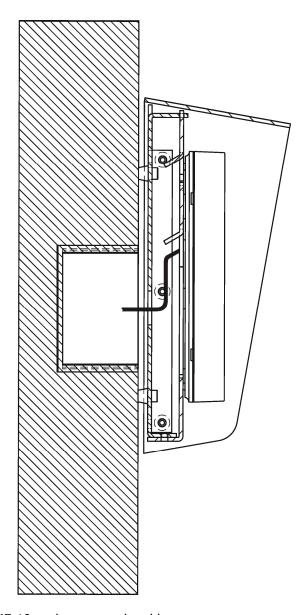
Fig. 4 Cable run in ME-10 enclosure panel and base
