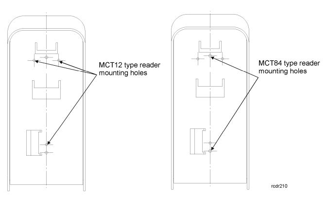
Fig. 3 Arrangement of mounting holes for MCT12 type and MCT84 type readers
