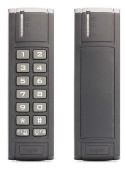
MCT12M series reader is outdoor identification terminal designed for use in the RACS 5 access control system. It enables identification of users by means of MIFARE® 13.56 MHz cards. Communication with the controller is carried out via a modified RS485 standard, which allows
