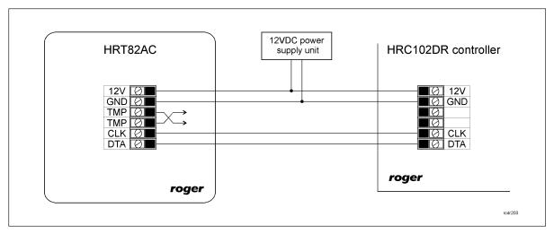
Fig. 3 Connection to controller without 12VDC power supply output
