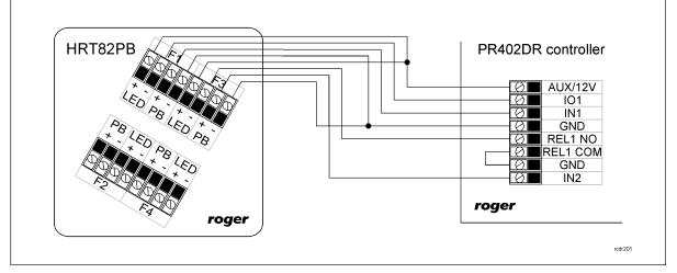
Fig. 2 Example of connection to PR402DR controller
