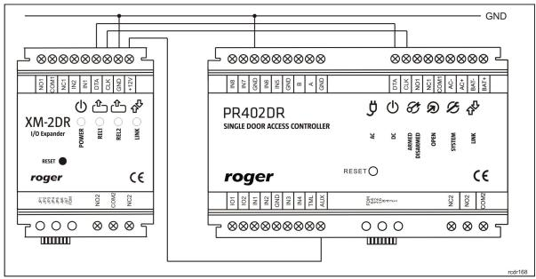
Fig. 2 Connection of XM-2DR expander with PR402DR controller
