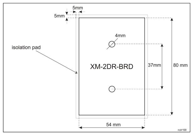
Fig. 3 The arrangement of XM-2DR-BRD mounting holes
