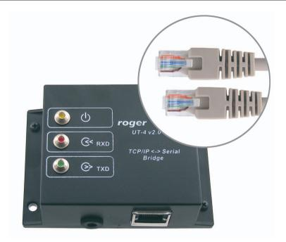
The UT-4 interface enables communication with various devices equipped with RS232 serial port trough a computer network. The device is equipped with serial port which can be configured as RS232, RS422 or RS485 and with 10/100 Mb/s Ethernet port for communication within computer network.
