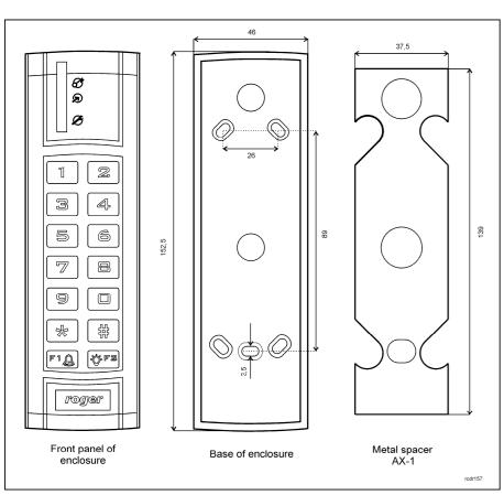
Fig.1 General view of AX-1 metal spacer
