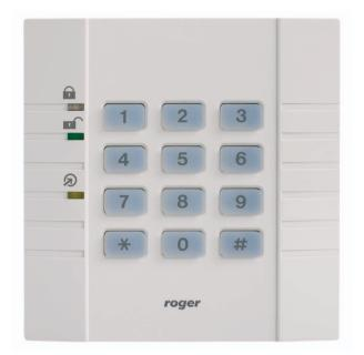
SL2000B code locks identify users through PIN codes. SL2000B locks offer possibility to program up to 55 different codes and are preferred to be applied in Access Control installations. In parallel to controlling access they can also control any device or the system requiring switching of turn-on/turn-off type.
