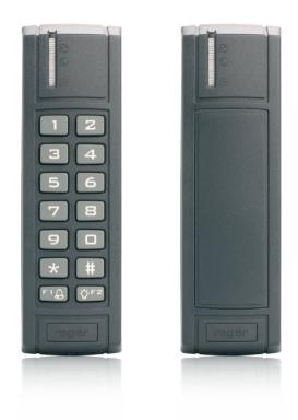
PR311SE access controllers are designed as popular and low cost access control solutions. They can be used either in standalone or integrated access systems for up to 1000 users. PR311SE units are equipped with RS485 interface which can be used for both programming and online communication in network system. Access control system based on PR311SE controllers can be managed locally through COM/USB serial port or remotely by computer network WAN/LAN (UT-4 interface required).
