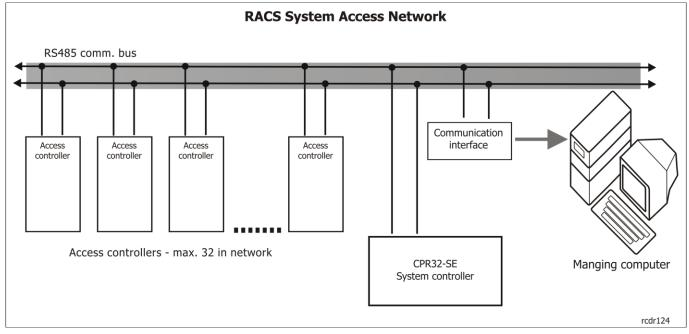
Generally, CPR32-SE works as centralized event buffer (250.000 events) and centralized clock for the entire access network. Also, it controls exchange of data between access controllers located within single access network which is necessary for so called "global functions" (e.g. APB Zones, Alarm Zones).
