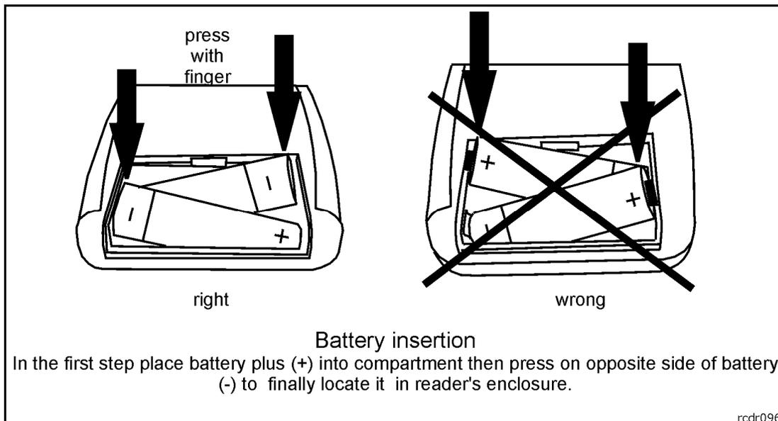
Fig.14 How to replace batteries in PATROL II LCD reader
