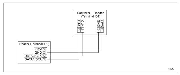
Fig. 4 Connection of Wiegand/Magstripe reader
