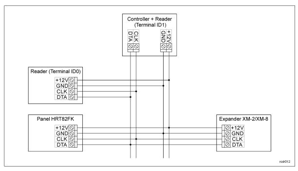
Fig. 3 Connection of PRT series readers, XM-2/XM-8 expanders and HRT82FK panel
