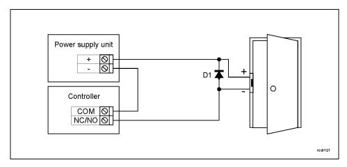
Fig. 2 Connection of door lock
