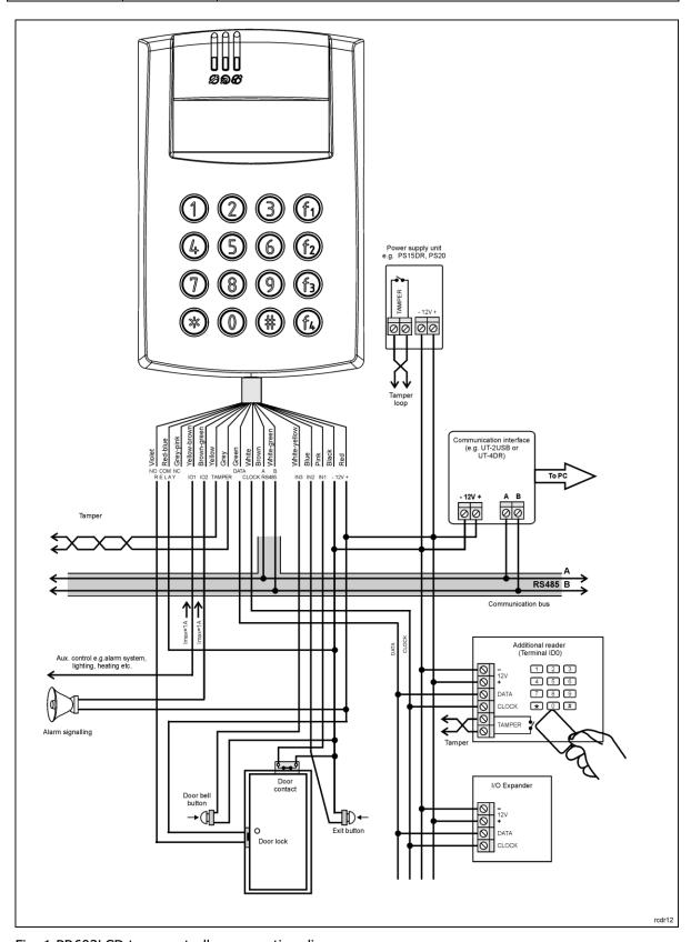
Fig. 1 PR602LCD type controller connection diagram
