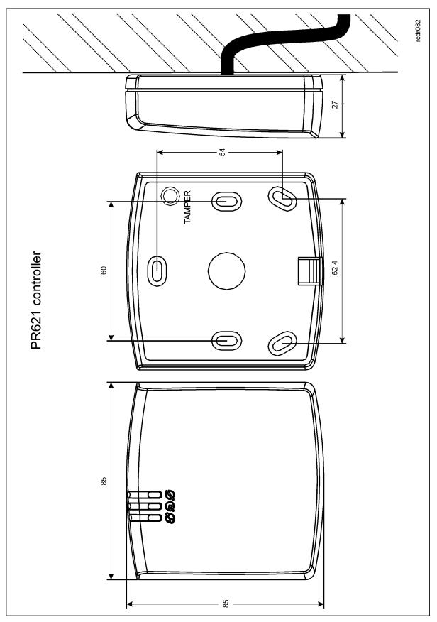
Fig. 4 Installation of PR621 controller
