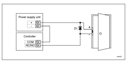
Fig. 2 Connection of door lock
