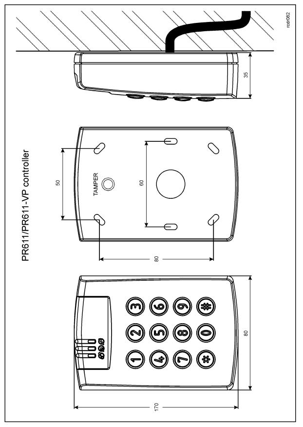
Fig. 3 Installation of PR611 controller
