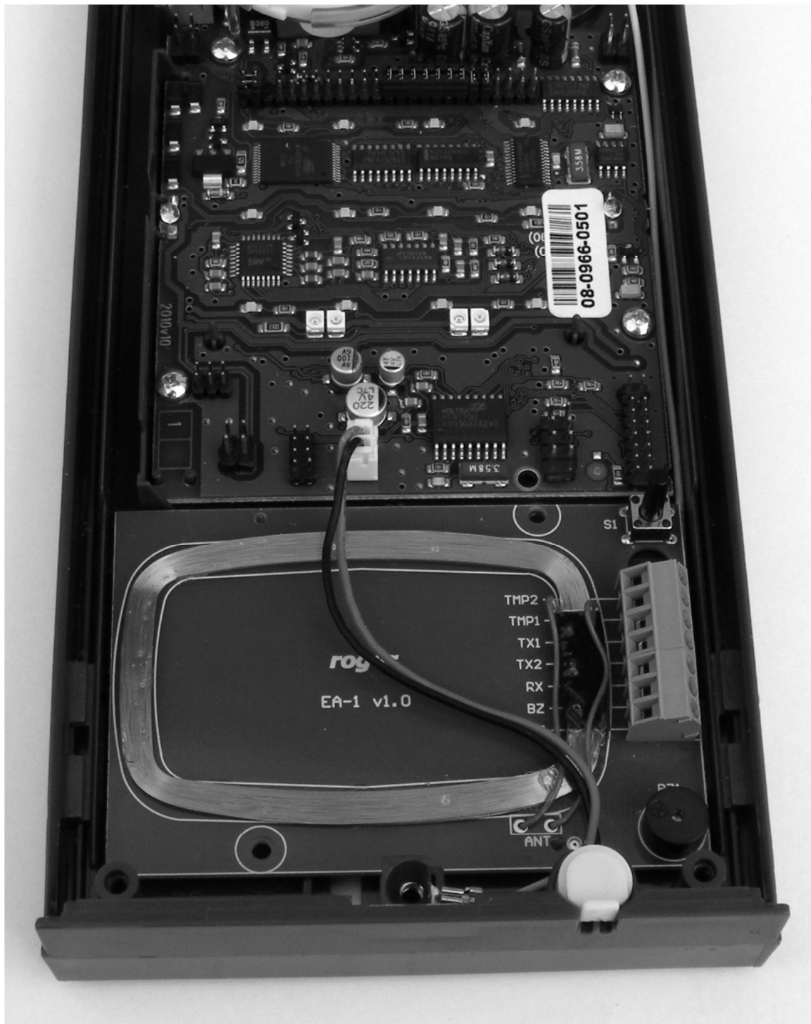
Fig.2 Installation of EA-1 module in HELIOS entryphone
