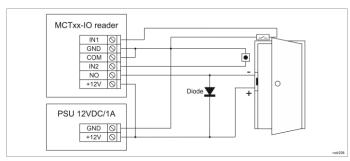
Fig. 6 Connection of door lock, door contact and exit button to MCTxx-IO terminal
