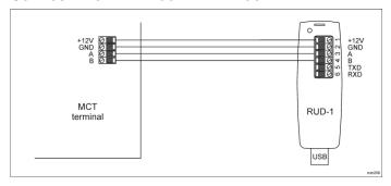
Fig. 1 Connection of MCT reader to RUD-1 interface.
