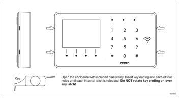
Fig. 2 Enclosure disassembly
