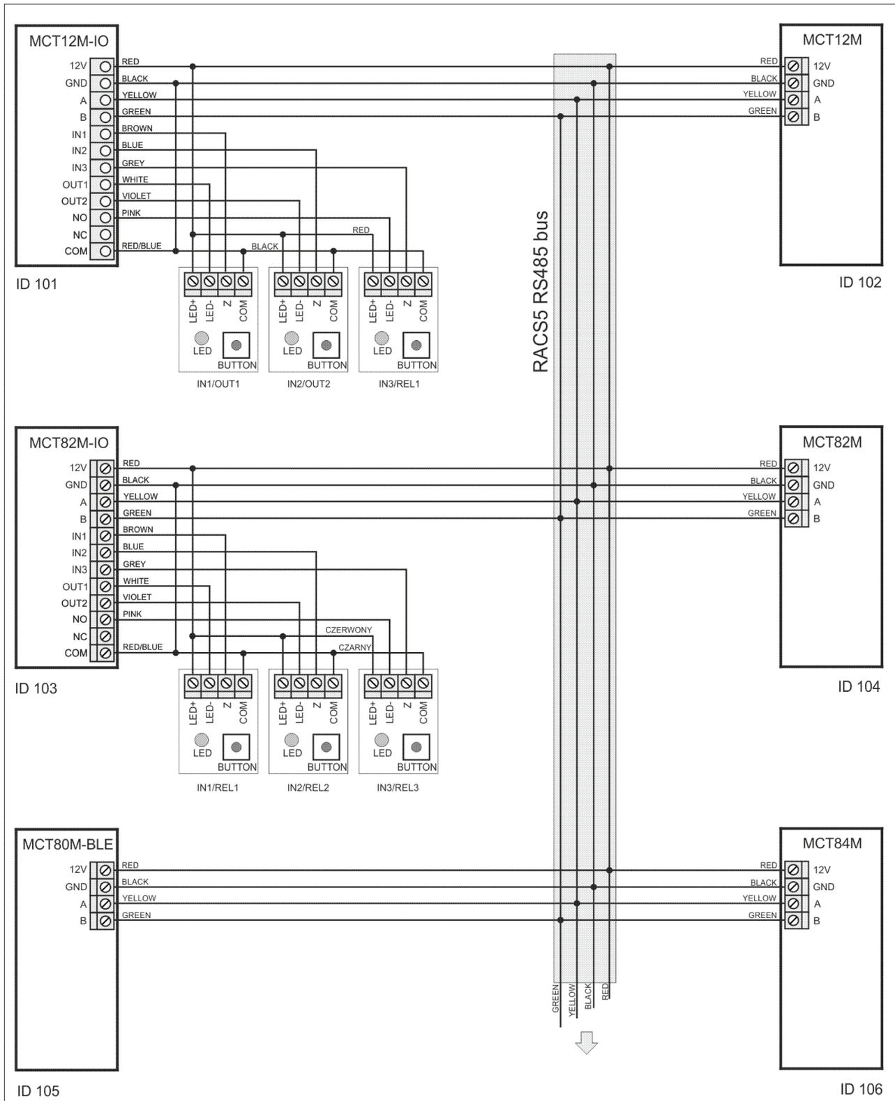
Fig. 2 DB-6A connection diagram 1/2
