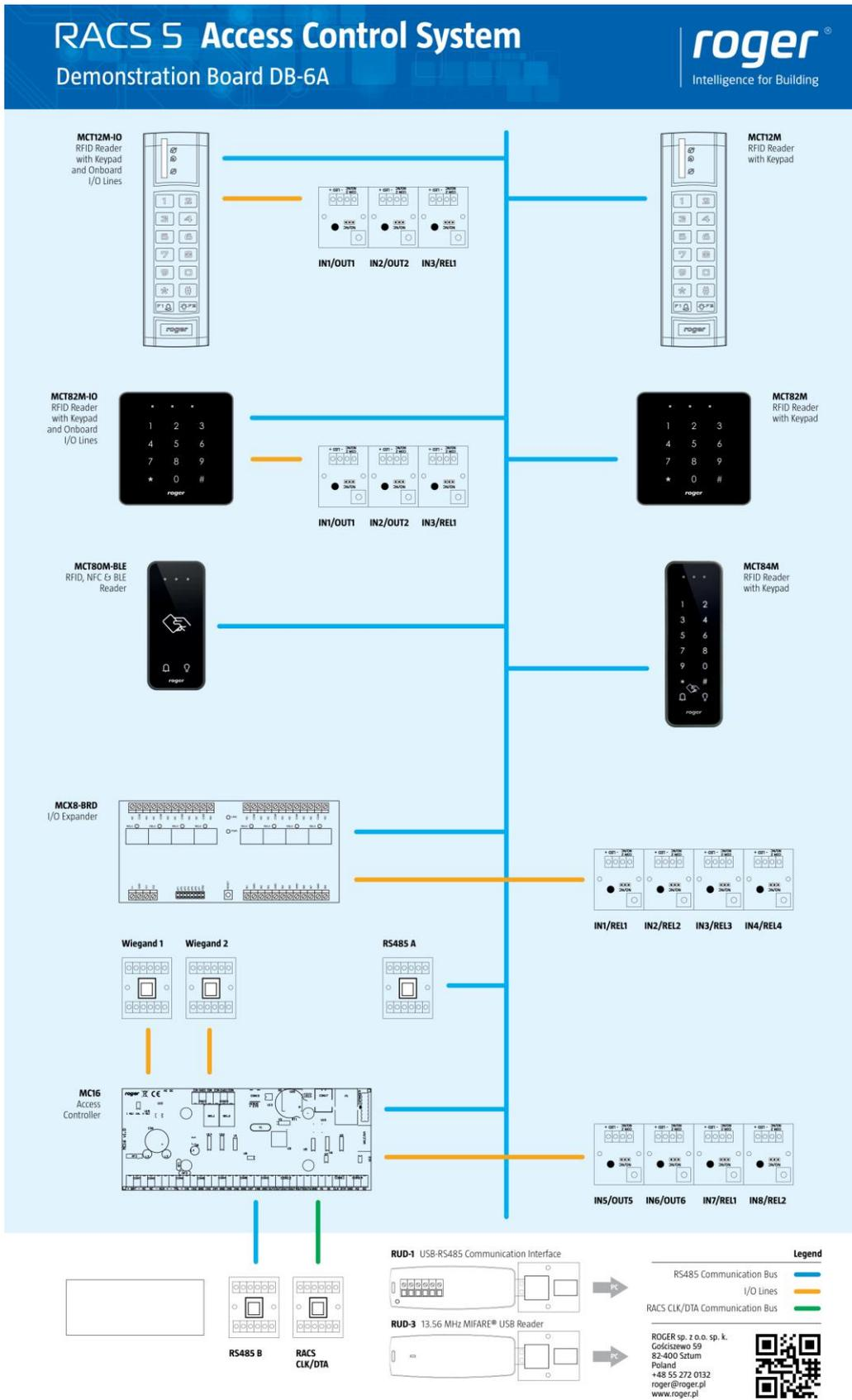
Fig.1 DB-6A functional diagram
