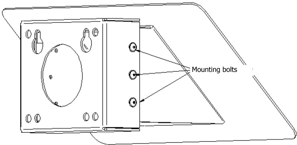
Fig. 2 Arrangement of front panel and base assembly holes
