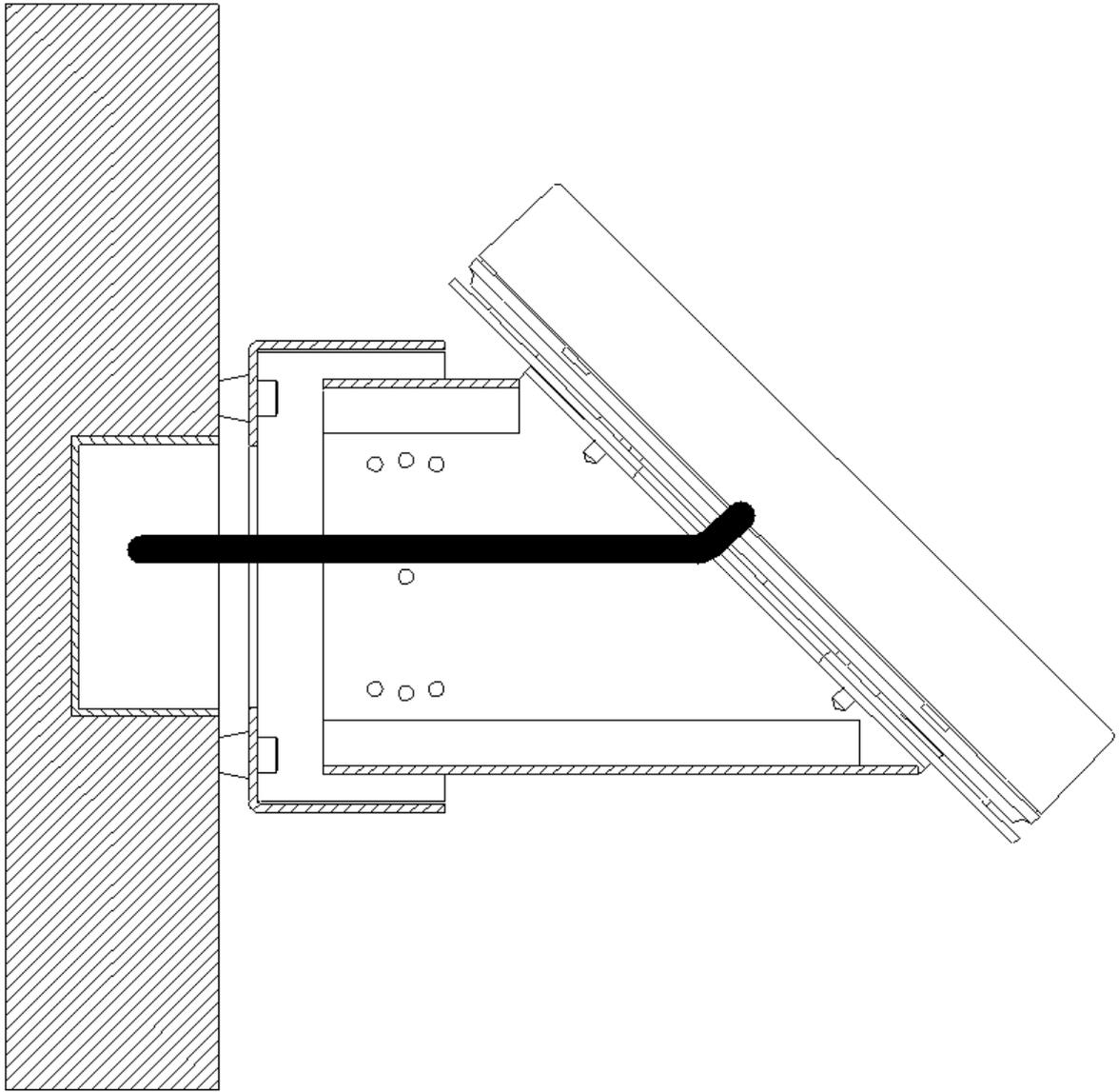
Fig. 4 Arrangement of connection cable
