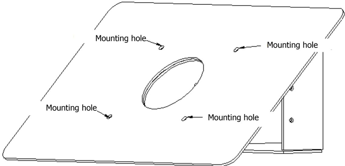
Fig. 3 Arrangement of MD70 mounting holes
