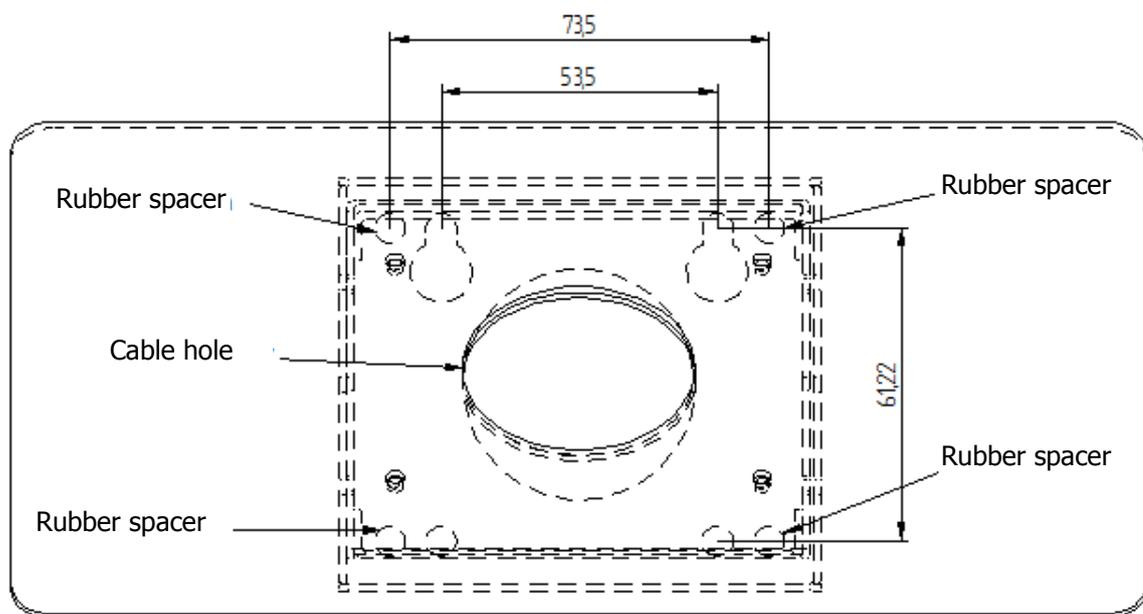
Fig. 1 Arrangement of wall mounting holes
