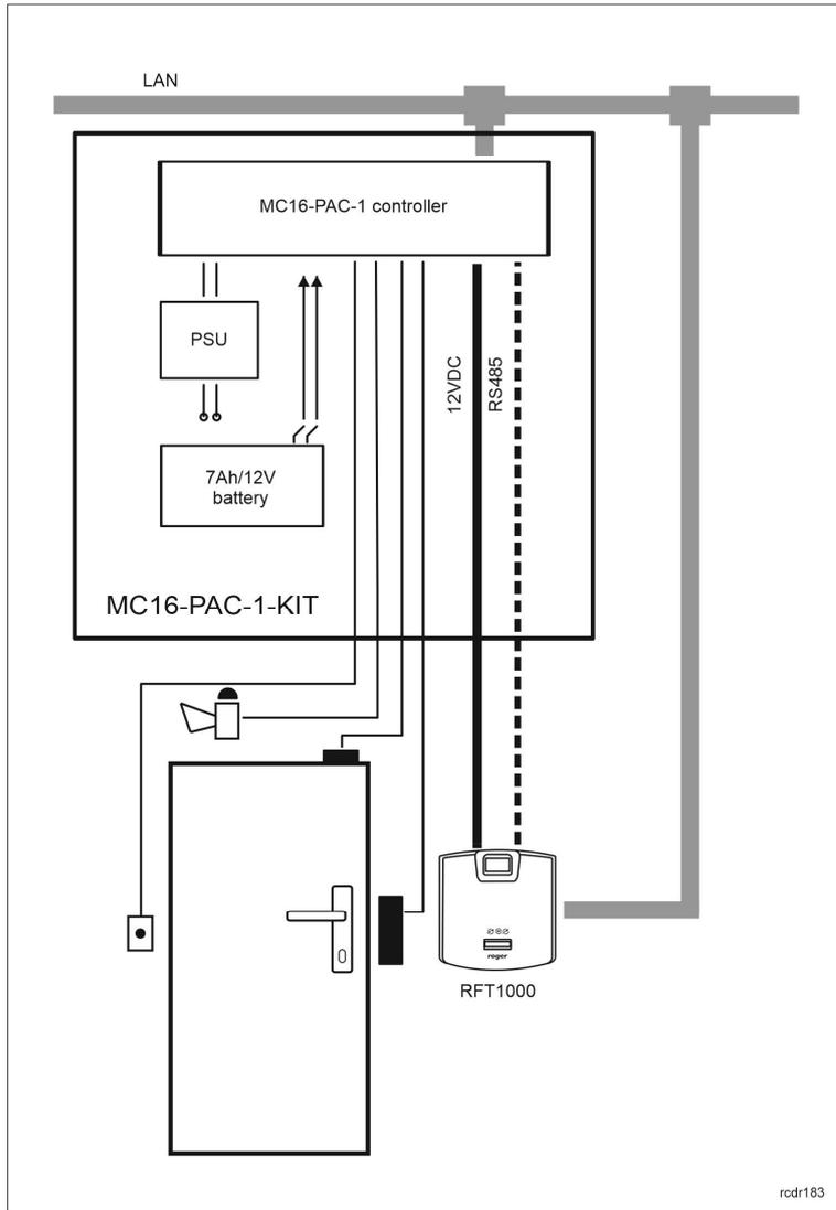
Fig. 1 The example of RFT1000 operation with MC16-PAC-1-KIT
