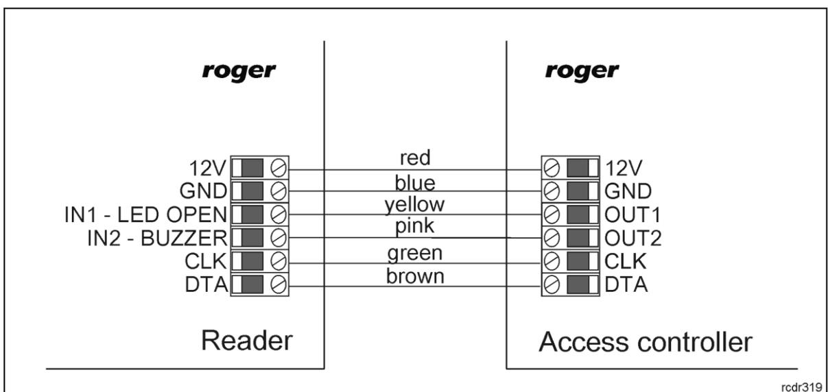
Fig. 1 Connection of reader to access controller (Wiegand)
