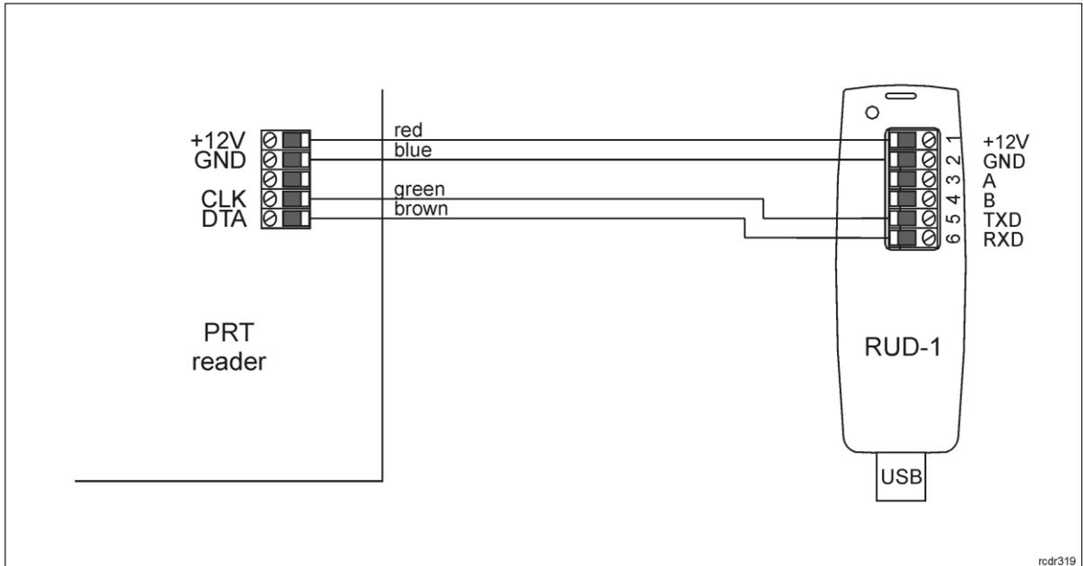
Fig. 3 Connection of reader to RUD-1 interface
