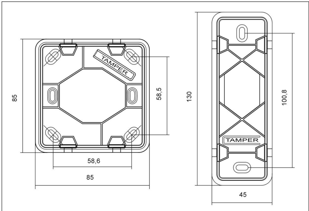
Fig. 9 Dimensions and tamper details
