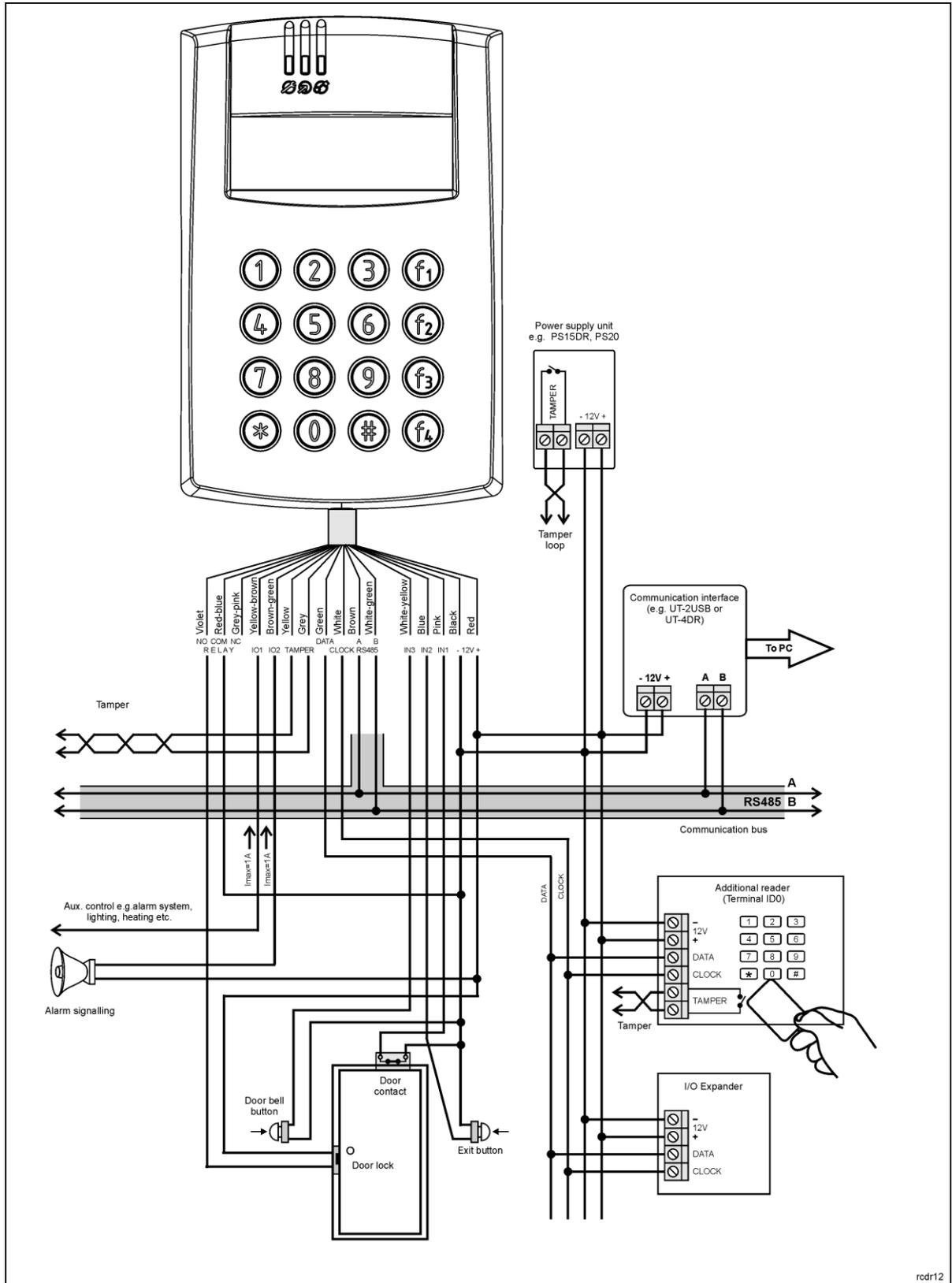
Fig. 1 PR602LCD type controller connection diagram
