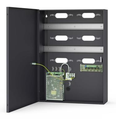
The ME-43-S enclosure is dedicated to RACS 5 modules and devices which require installation on DIN rail along with 17 Ah battery. The enclosure is equipped with 2 DIN rails, buffered power supply 13.8 V/4 A, tamper contact and main fuse switch. Access to the internal space of
