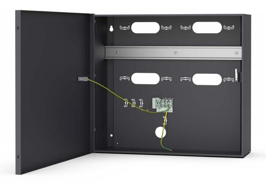
The ME-40 enclosure is dedicated to RACS 5 modules and devices which require installation on DIN rail along with 17 Ah battery. The enclosure is equipped with one DIN rail, tamper contact and mains fuse switch. Access to
