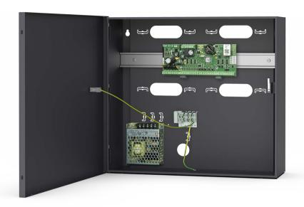
One-door access control kit for the RACS 5 v2 ST system. The kit comprises a metal enclosure with a power supply and a network access controller. MC16-PAC-ST-1-KIT enables the implementation of read-in/read-out access control for one door using RS485 (MCT series readers), RACS CLK/DTA (PRT series readers) or Wiegand readers.
