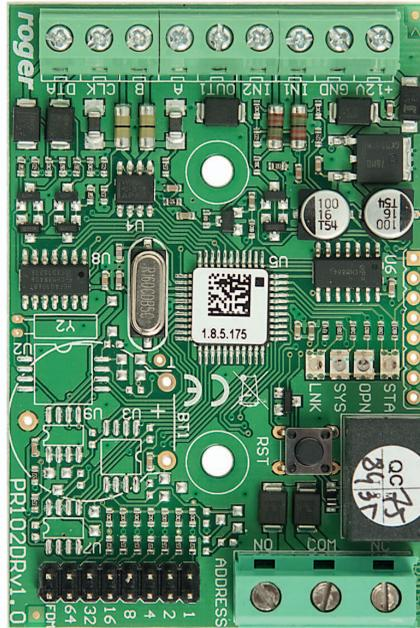
MCX102-BRD is I/O expander dedicated to RACS 5 system. Expander offer two NO/NC input lines as well as one relay and one transistor output.
