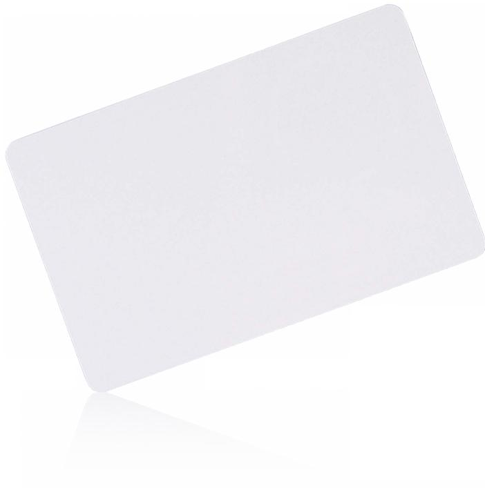
EM 125 kHz ISO size thin PVC proximity card with Q5 chip, EEPROM 264 bits, the card number (CSN) can be programmed by any PRTxxEM series readers running under RARC software (Windows), card can be used with PVC printers, photo ID pictures and text printing possible.
