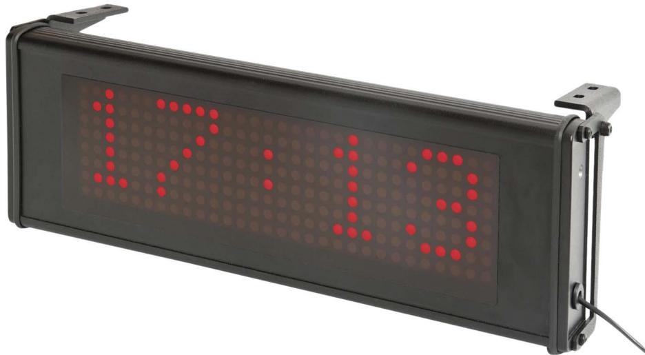
The ASCD-1 is a five segment LED matrix display. In RACS 4 the device can display system time in 24h format while in RACS 5 it can additionally display system text messages with maximal length of 32 characters. When the text is longer than matrix (5 characters) then it is smoothly scrolled. Alternatively the ASCD-1 can be used beyond RACS systems as a standalone clock using internal RTC or as a display presenting received text messages. The device can additionally display ambient tempe-
