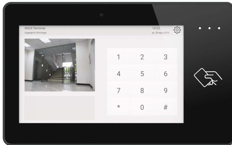
The MD70 is a graphic touch panel with a built-in camera and proximity reader. The device is dedicated to use in the RACS 5 access control and building automation system as a user identification terminal and a control panel. In particular, the panel can be used as a time and attendance (T&A) terminal. Users can log on to the panel via proximity cards, PIN codes, and QR codes. A built-in camera enables the recording of pictures of
