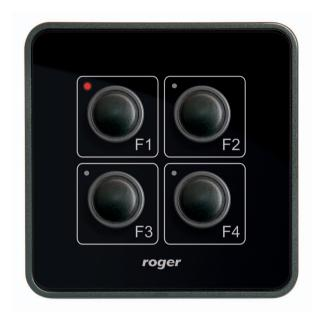
HRT82PB panel provides four momentary type buttons with insulated NO contacts and four externally controlled LED indicators. The NO contact can be used to trigger controller's input while LEDs to indicate state of controller's outputs. Panel can be used in other scenarios as long as its nominal electrical condition is assured.
