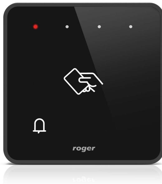
HRT82MF operates as a hall reader and besides providing access control it is equipped with a touch button for door bell and LED indicators to signal hotel staff presence in the room and such hotel services as assistance, make up room, do not disturb. Each state is signalled
