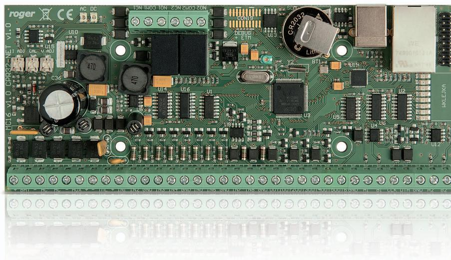
CPR32-NET-BRD network controller expands functionality of RACS 4 system and due to the built-in Ethernet interface allows for management of the access control system through LAN or WAN network. The most important features provided by CPR32-NET-BRD are: centralized event buffer, centralized clock and calendar, global
