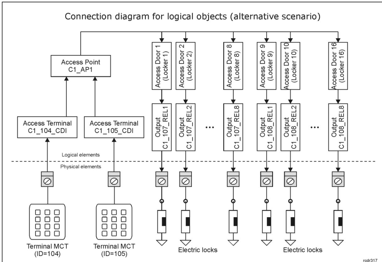
The difference between two above logic diagrams is such that depending on user Authorisations, in the first scenario each terminal can be used to control its 8 lockers while in the second scenario each terminal can be used to control any of 16 lockers. In the second scenario more than one Access Terminal (physical reader) is assigned to Access Point (logical reader). In this application note the first scenario is described.
