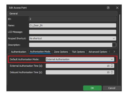
• In the same window with Access Points select *Add* to create Access Point to be operated as authorisation approval terminal. Name the point and close the window with *OK* button.
