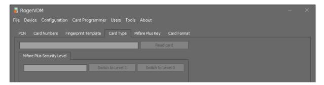
Security level can be changed only upward. On the level SL=1, MIFARE X Plus emulates MIFARE Classic card and then its programming is done as if it was MIFARE Classic card. When switched to SL=3 then it can actually be programmed and read in RACS 5 system as MIFARE Plus card enabling its security and functionality to be used in full extent.
