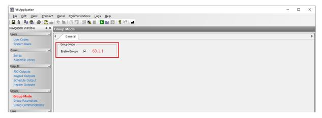
In this window the operator can enable Groups. The integration is based on association of Alarm zones from RACS 5 system with Groups (Alarm zones) from Galaxy systems. If Groups with their Zones (detectors) are not defined then within the integration it will not be possible to arm/disarm particular detectors but only all detectors.
