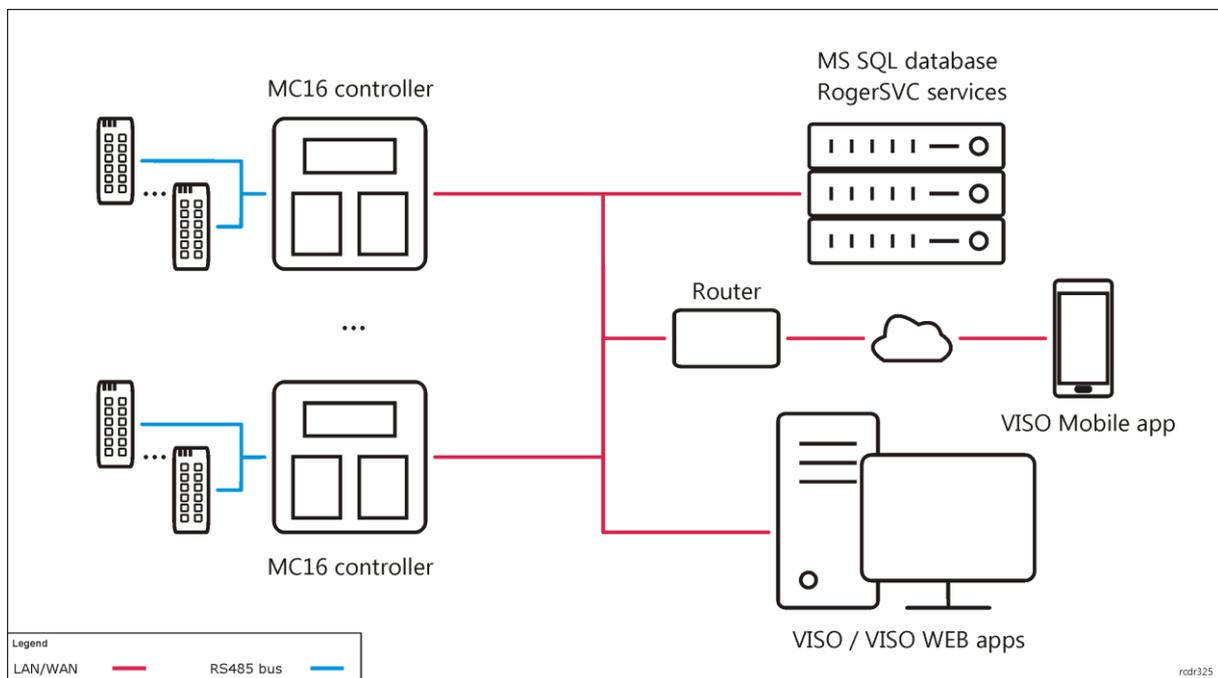
Note: In principle, the MC16 controller can be used in both WAN and LAN, while the manufacturer's warranty is covered only by working in an isolated LAN reserved exclusively for the access control system in which the controller is to be used.
