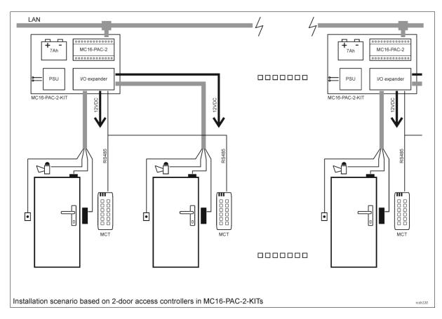
MC16 controller kits for three doors (MC16-PAC-3-KIT) and four doors (MC16-PAC-4-KIT) include expanders with more I/Os (MCX4D instead of MCX2D), power supplies with greater current (PS4D instead of PS2D) and larger metal enclosures with space for 7-17Ah batteries. Nevertheless their installation scenario is similar to installation of controller kit for two doors (MC16-PAC-2-KIT).
