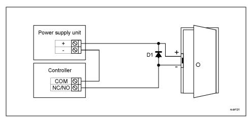
Fig. 2 Connection of door lock
