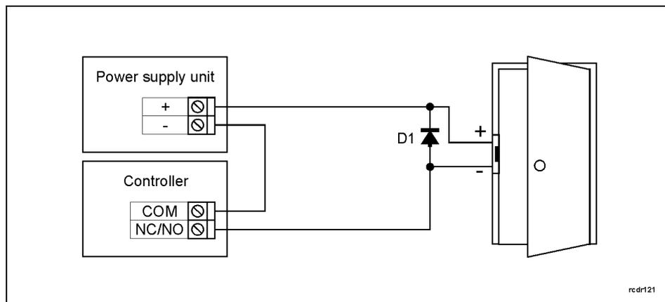
Fig. 5 Connection of door lock
