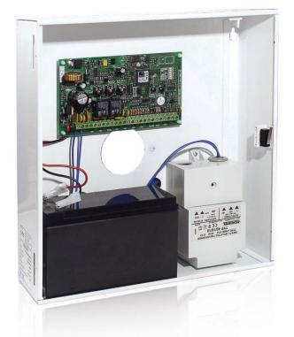
CPR32-SE module with power supply and battery installed in a metal enclosure
